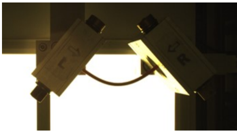
Figure 1: Left: Top-view of MeSOMICS [3] bending experiment. Right: Schematic representation of experimental procedure for MeSOMICS bending measurements. At the left clamping point, horizontal displacements are stepwise applied, resulting in different bending configurations. At the right clamping point, the resulting horizontal reaction force is measured.
