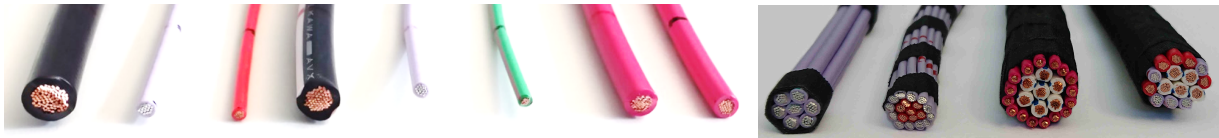
Figure 1: Examples of single cables (left) and cable bundles with different taping patterns (right).
